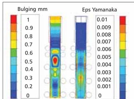
**Fig 1** Simulation using Thercast made it possible to establish the mathematical relationship between the bulging of the outer skin of the continuously cast bloom (left) and the Yamanaka criterion (Graphics : Ascometal)
