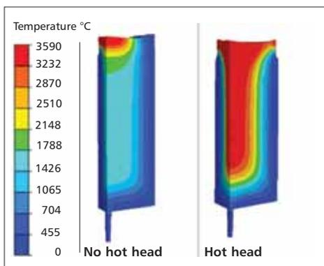
**Fig 10 Use of Thercast when optimising pouring parameters: influence of ingot head insulation on the macro segregations in an ingot with rectangular cross section**
