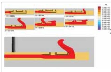
**Fig 8 Analysis of the filling process of a flat ingot using simulation software (Graphics: Industeel)**
