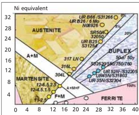
**Fig 7 Steel grades produced by Industeel (Graphics: Industeel)**
