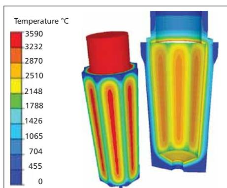
**Fig 11 Prediction of temperatures in an octagonal ingot as well as in the related mould (right) using Thercast**
