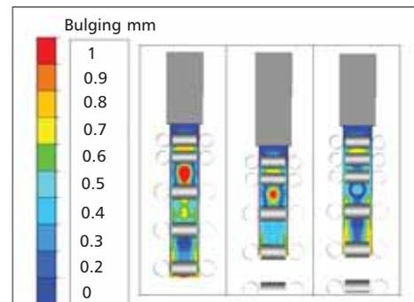
**Fig 2** Analysis of the possible modifications to the continuous caster to prevent bulging of the strand: initial situation (left), use of an elongated mould (centre) or installation of an additional support roll below the mould (Graphics: Ascometal)
