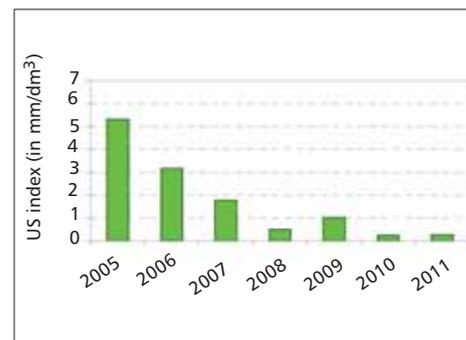
**Fig 5** Reduction of the internal defects detected in rolled wire rod using ultrasonic testing (10MHz) over a period of seven years (Graphics : Ascometal)
