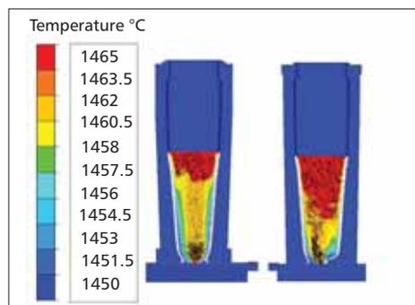
**Fig 4** Visualisation of the melt flow velocity speeds and directions and temperature profile in a half-filled bottom pored ingot mould for two different diameters of the runner channel (Graphics: Ascometal)
