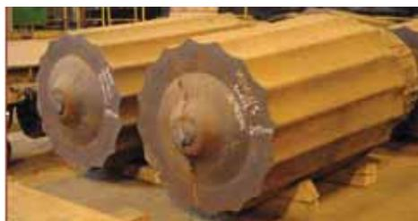
**Fig 6 Industeel produces cast ingots in nearly 50 different sizes weighing between 2t to 300t by bottom pouring (Photos: Industeel)**
