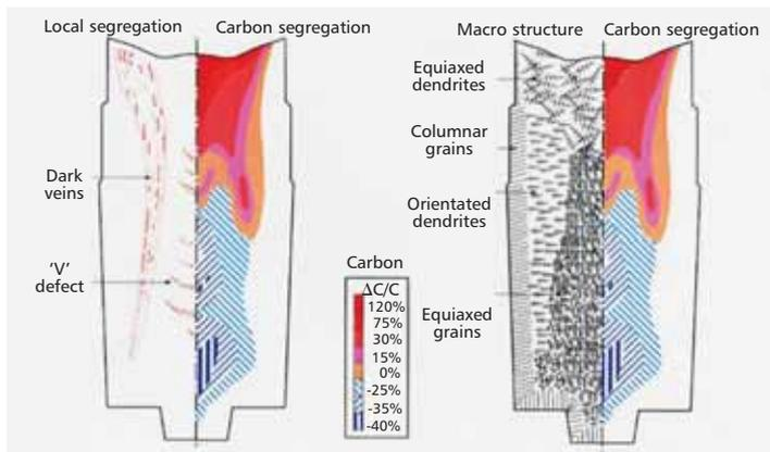
**Fig 9 Prediction of macro segregations and the structure of an ingot**
