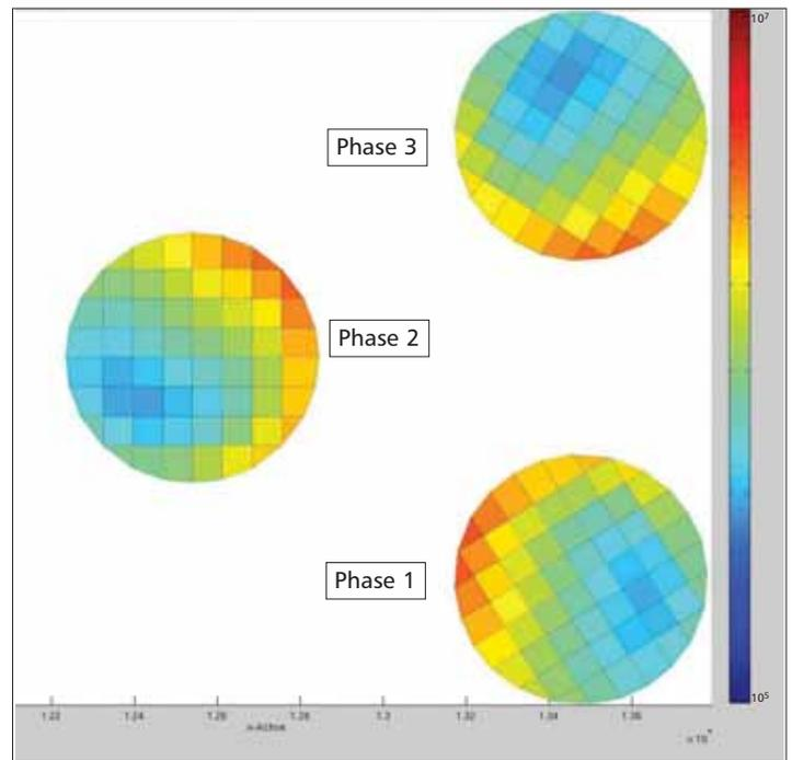
**Fig 5** Current density distribution in the three electrodes at cross sections selected at the mid-length of each electrode
