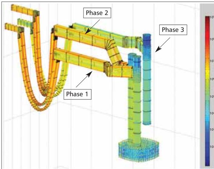
**Fig 6 Three dimensional current density distribution at one-phase short circuit calculation (only phase 1 and 2 are carrying current) Log scale: (blue)  $1 \times 10^2$  A/m<sup>2</sup> –  $1 \times 10^9$  A/m<sup>2</sup> (red)**
