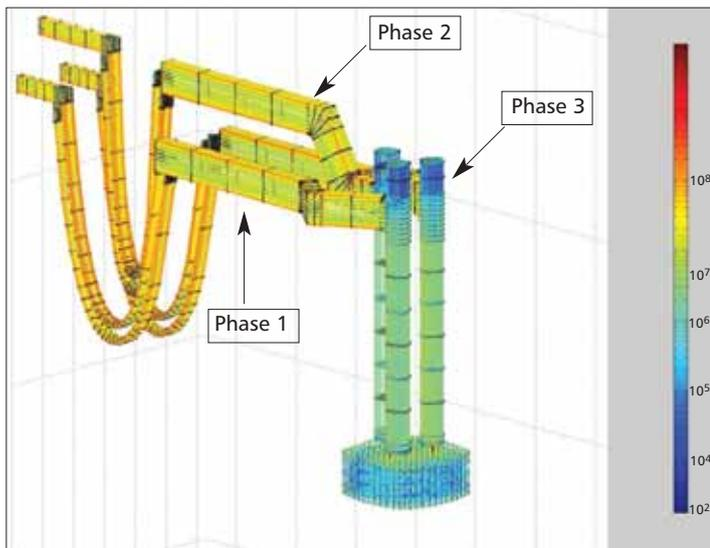
**Fig 1** Three dimensional current density distribution of the calculated furnace
