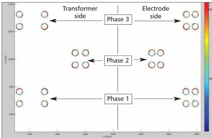
**Fig 4** Current density distribution in the four flexible cables per phase; section parallel to electrode arms below the connection of cables with conductors and electrode arms (left transformer end; right electrode end)
