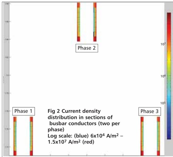
**Fig 2** Current density distribution in sections of busbar conductors (two per phase)
