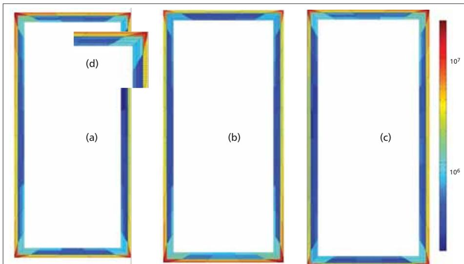
**Fig 3 (a-d)** Current density distribution in cross-section of each electrode arm at similar locations. Log scale: (blue)  $1 \times 10^5$  A/m<sup>2</sup> –  $2 \times 10^7$  A/m<sup>2</sup> (red)
