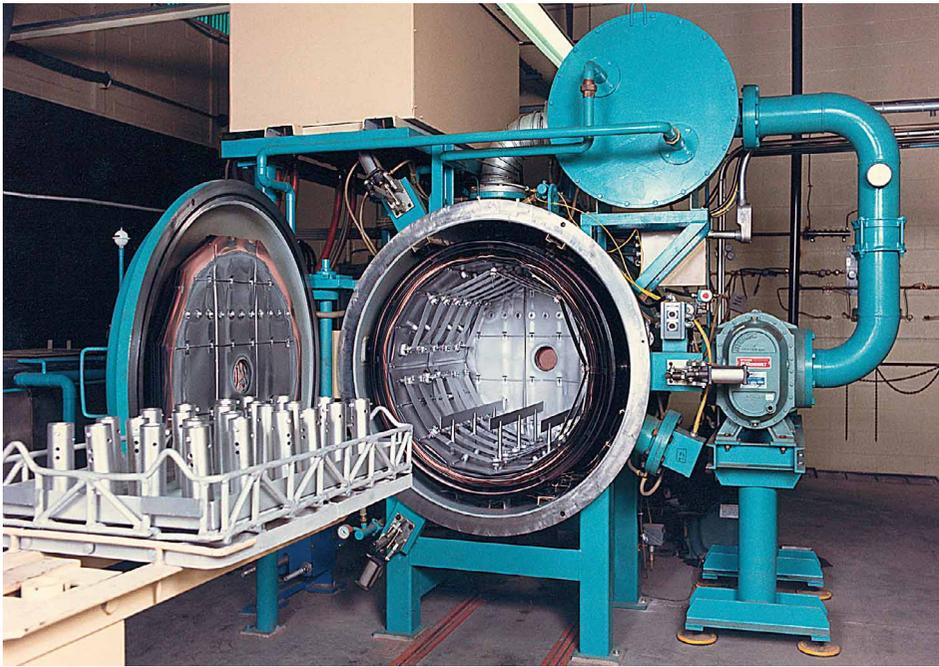
Parts loaded into a VAC AERO VAH2636 vacuum furnace for vacuum hardening
