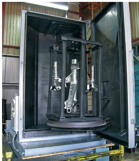
Parts washer used to remove machining residue prior to vacuum heat treating
