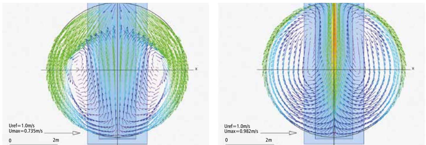
Fig 2. Melt flow velocity vectors simulated in a 100 ton spout tap EAF<sup>[2]</sup>
