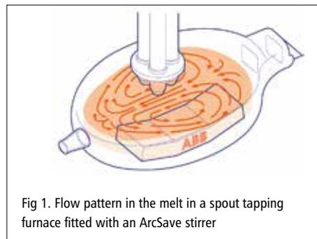
Fig 1. Flow pattern in the melt in a spout tapping furnace fitted with an ArcSave stirrer
