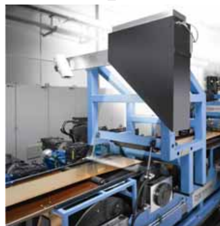
The monoblock version showing separate camera (top left) and beam projector (top right)
