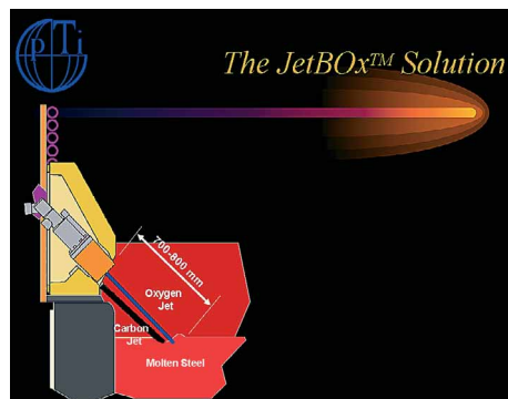
Fig 1 Principle of the JetBOx™ sidewall injection system
