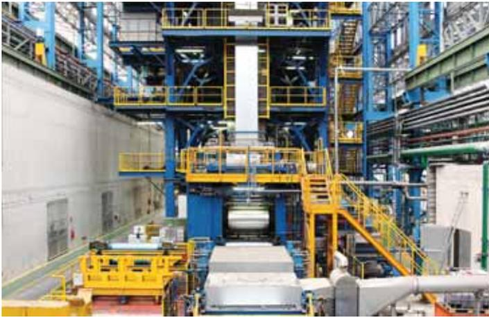
Marcegaglia Ravenna operates four hot dip continuous galvanising lines, one a combi line for organic coating
