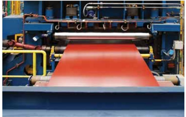
Strip pre-painted on the combi galv+paint line is rapidly cured using near infra-red technology
