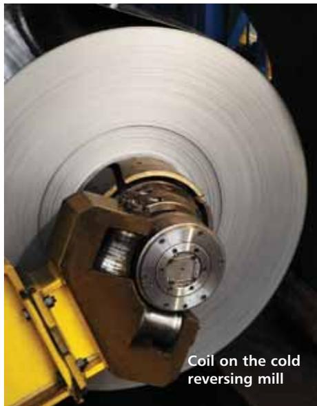
Coil on the cold reversing mill
