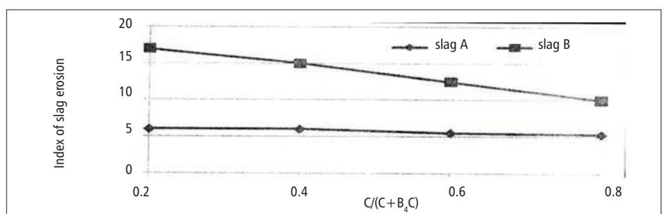
Fig 14. Relation between C/(C+B<sub>4</sub>C) and index of slag corrosion
