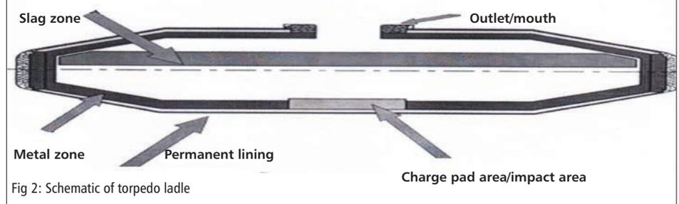
Fig 2: Schematic of torpedo ladle
