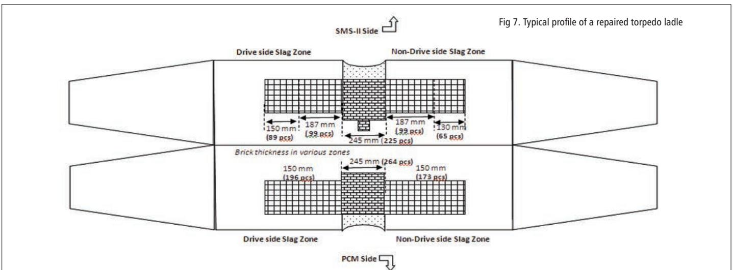
Fig 7. Typical profile of a repaired torpedo ladle
