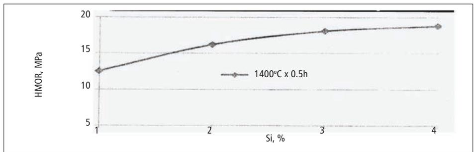
Fig 11. Relation between silicon addition and HMOR
