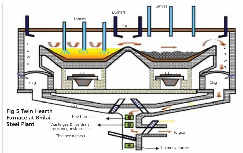
**Fig 5 Twin Hearth Furnace at Bhilai Steel Plant**
