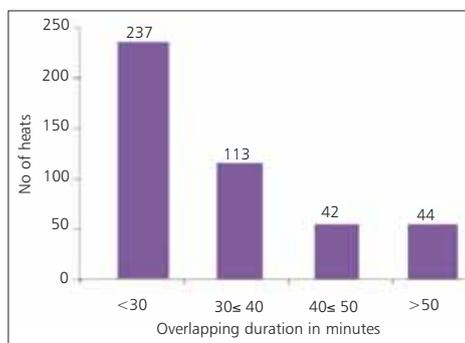
**Fig 6 Restriction of oxygen blow overlap duration to decrease gas load on roof**
