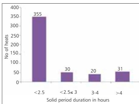
**Fig 7 Reduction in charging time for solids to reduce overcooling of roof bricks**
