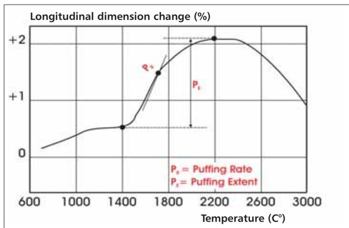
**Fig 4 Dilatometry curve during graphitisation**
