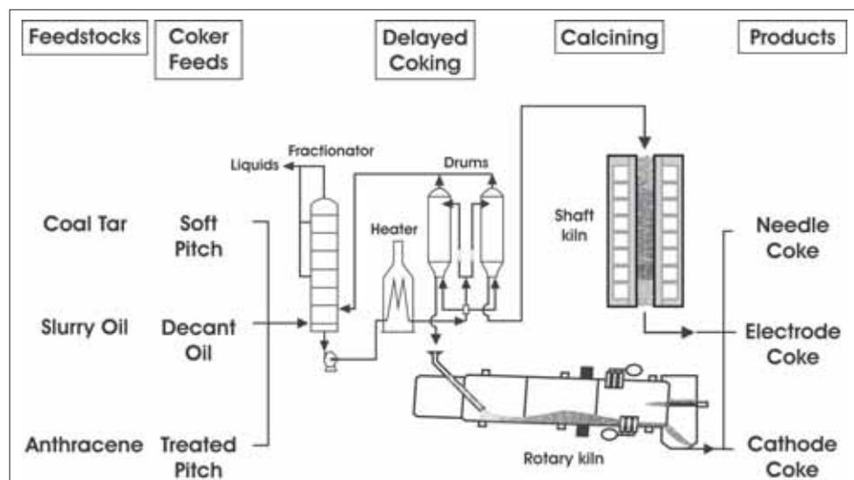
Fig 1 Production of Needle, Electrode and Cathode cokes
