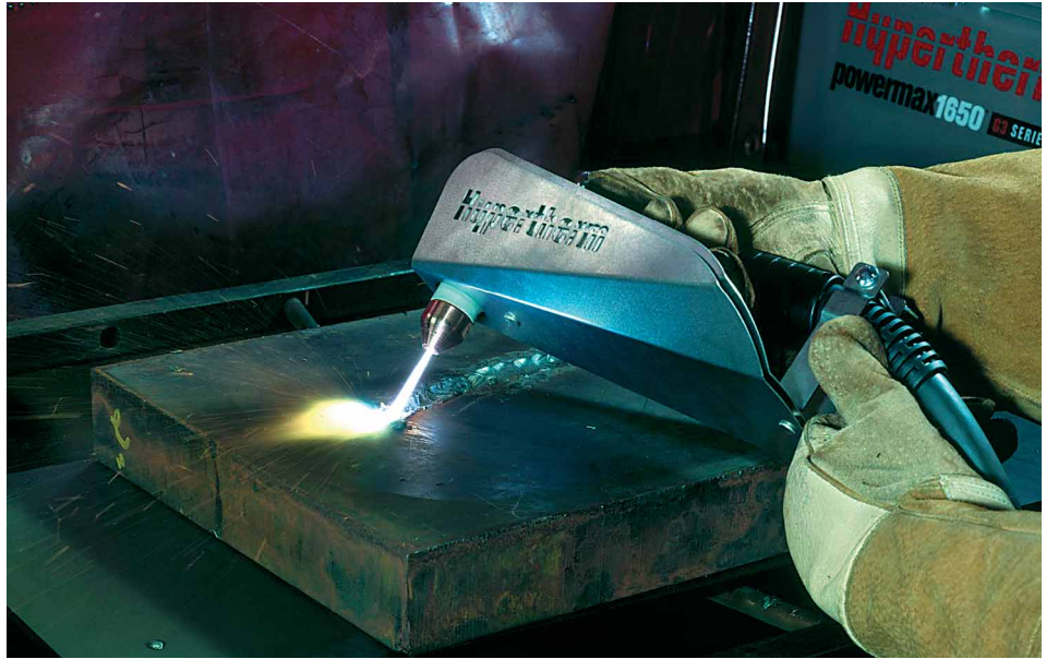
Small, portable systems are effective gouging tools
