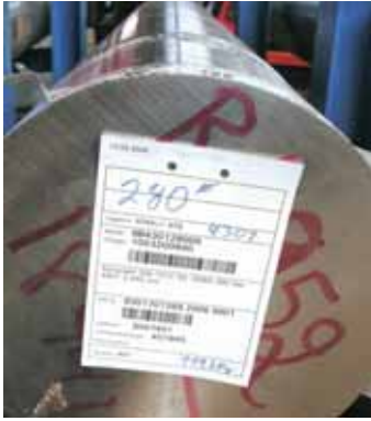
Fig 2 Labels are machine printed and placed outward in the racks
