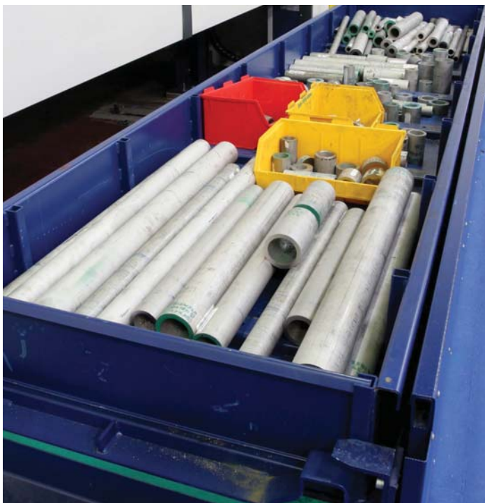
The base of a special 5-tonne-capacity cassette is raised hydraulically to enable billets to be offloaded by hand pallet truck.
