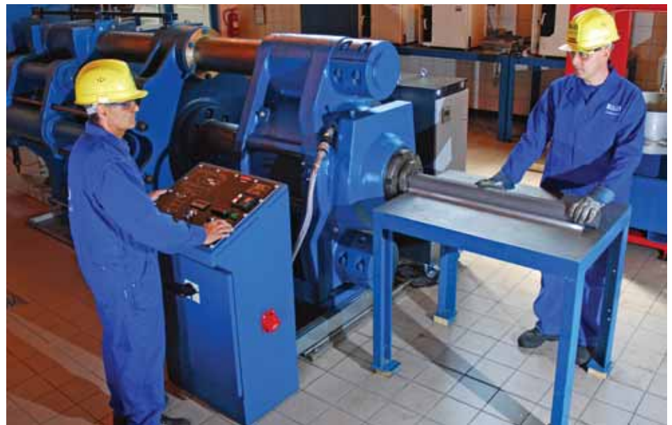
Fig 3 Pilot plant to prepare dry aggregate, and 400t extrusion press
